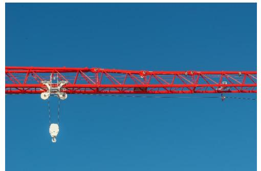
The transition of the jib sections in 4-chord design to the jib sections in 3-chord design. On the right, the hoist rope support, which reduces the rope slack from the standard 10 meters to only 1.5 meters.
