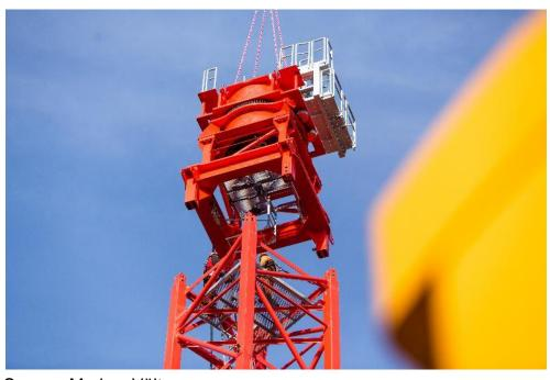
The WOLFF 8076 Compact has a tower connection for the 2.90 x 2.90 meter TV 29 tower element.
