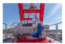
Easy maintenance, efficient warehousing: Identical winches are used for the hoisting and luffing gears. The latter is positioned at the bottom of the tower top and can therefore be accessed very conveniently.
