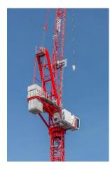
More comfort, more safety: The hoisting gear is positioned on the jib. This makes it possible to reeve the hoisting rope and completely pre-assemble the jib on the ground.
