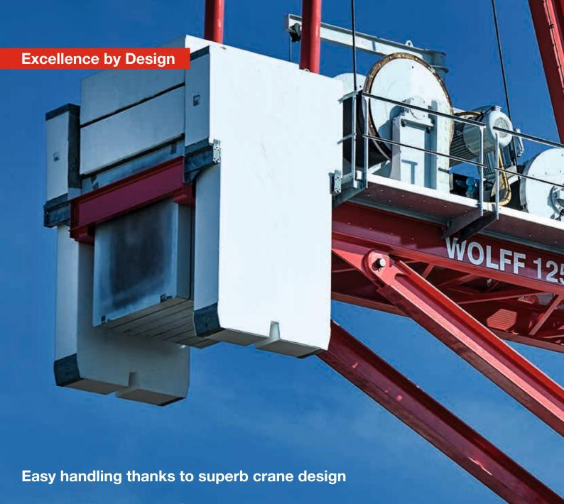
Despite its XXL lifting capacity, the WOLFF 1250 B is designed according to the same modular principle as all WOLFF tower cranes, with a focus on keeping individual component weights down to facilitate assembly and transportation.
