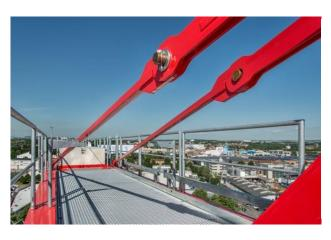
The counter jib with support beams for the easy positioning of the bracing rods and with transport aids. Also, the new WOLFF 6020 *clear* features more galvanized parts, such as railings, platforms and covers, as well as specially coated bolts to prevent corrosion.
