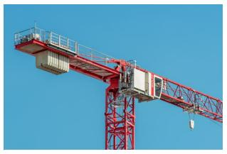
The counterweights are no longer included as standard in the basic crane package or the jib extensions. The customer can use counterweight blocks from his existing WOLFF fleet, or buy these separately as required, which is a decisive advantage economically seen.
