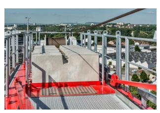
The counter jib has been fitted with new railings that are suitable for attaching safety harnesses thus improving the safety for technicians working on the counter jib.
