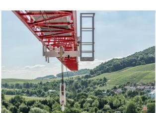
WOLFF engineers redesigned the trolley by replacing the rollers with wheel flanges used to date by rollers without wheel flanges and a new guide roller on the jib, thus optimizing the run of the trolley.
