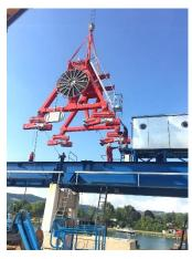
The 145-ton operating weight of the crane had to be evenly distributed over 16 wheels, four wheels at each corner of the undercarriage.
