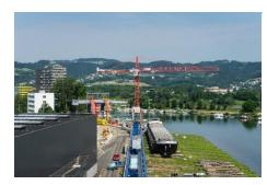
The WOLFF 7532.16 cross is used for moving ship dollies and performing maintenance work of the riverboats. Travelling on rails tremendously increases its working radius.
