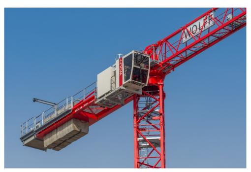
The WOLFF 7021 Clear can be individually equipped according to customer needs and budget. In the version with a divisible lower part of the top, as shown here, the assembly weight of the tower top section can be reduced to up to 6.4 tons. A more cost-effective, non-divisible lower part of the top is available for price-sensitive customers.
