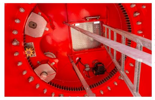
Significantly reduced maintenance effort is also promised by the standard central lubrication of the slewing connection and optionally of the tooth flanks. A lubrication pinion (yellow) can be installed upon request for precise lubrication and accurate distribution of lubricants.
