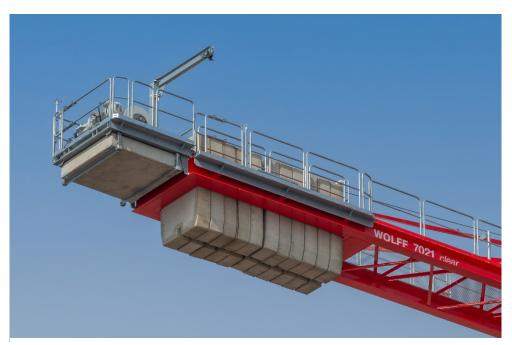
The redesigned ballast frame for the hoist winch can be easily assembled and removed for transport thanks to a quick connection. The railings have also been redesigned. They are lighter and remain in place during transport. The optional auxiliary crane at the hoisting gear facilitates maintenance.
